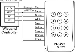
To change the status LED colour from violet to green apply a negative signal (0 to 2V) to the Yellow wire or a positive signal (2.5 to 28V) to the Blue wire.
